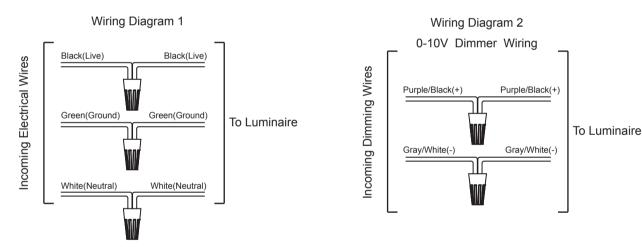
7) Check the wiring, make sure everything is correct. Recover the connection box. Then turn on power to light up the luminaire.
